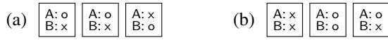
Fig. 1. Two ways of voting for the second candidate (candidate B) in the ThreeBallot protocol, where x represents a marked position and o represents an unmarked position. All the other possibilities of voting for B can be obtained as permutations of these two.
