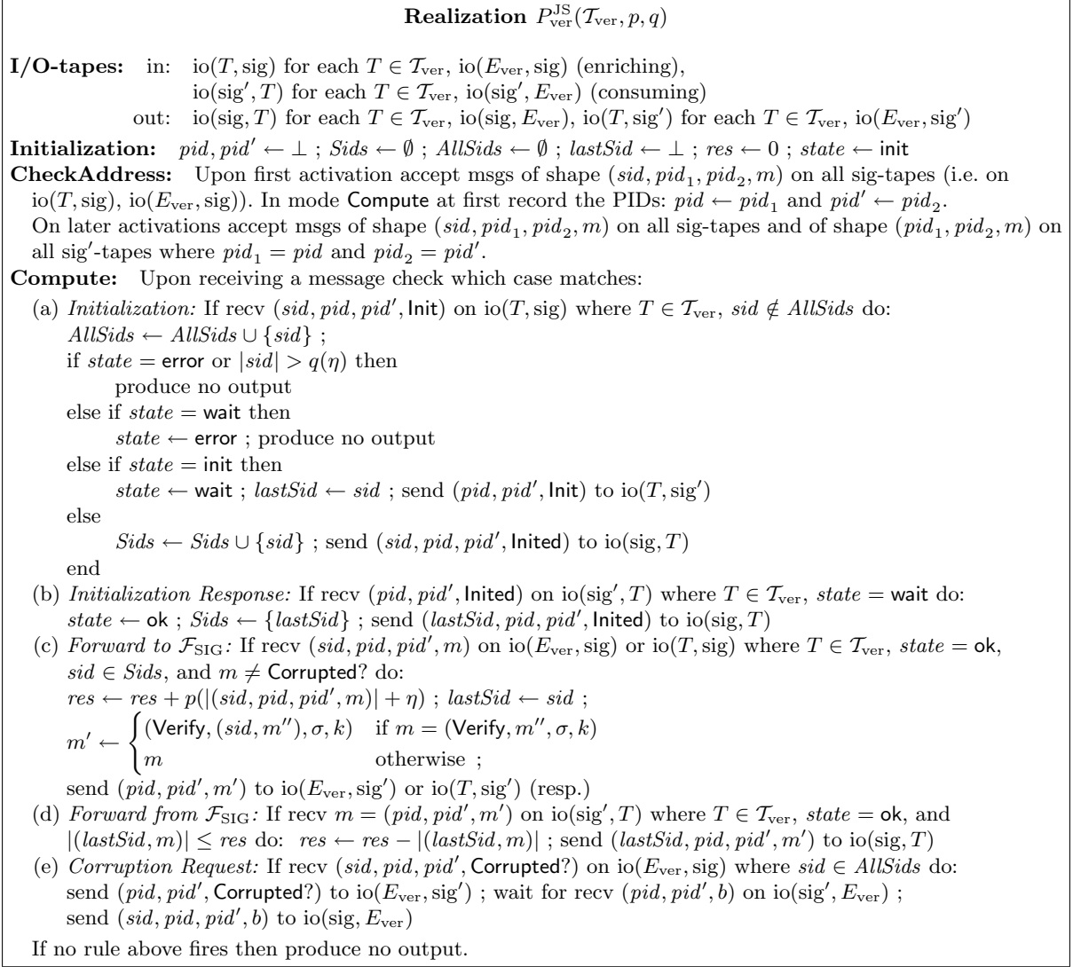
Fig. 11. Joint state realization \mathcal{P}_{\text{SIG}}^{\text{JS}} = P_{\text{sig}}^{\text{JS}} | P_{\text{ver}}^{\text{JS}} for digital signature schemes, the verifier's part P_{\text{ver}}^{\text{JS}} .
